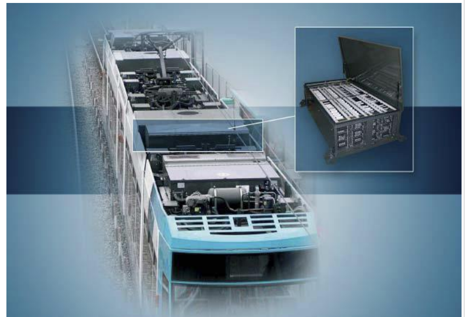
MITRAC Energy Saver (Bombardier) 2003 SuperCap 450 kg, 1 kWh [24]
